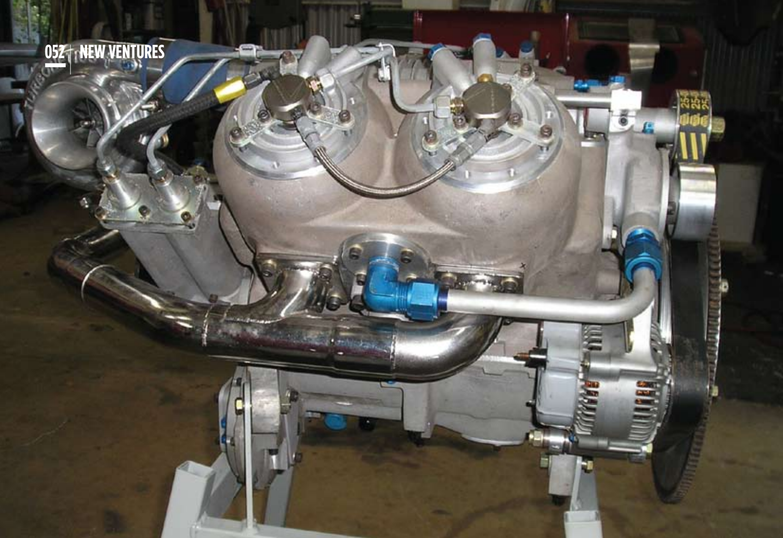
above: The Delta Hawk diesel engine lies at the heart of the D2 project.
